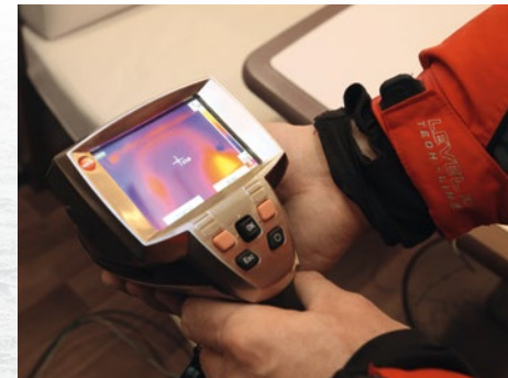
Checking the temperatures with a thermal imager
