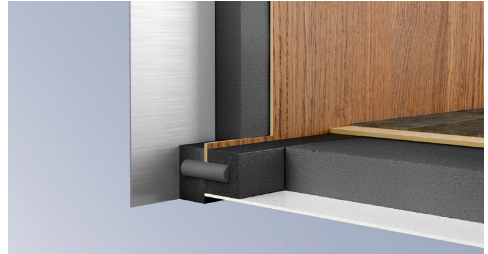
Well insulated: wall thickness 34mm, floor thickness 42mm
